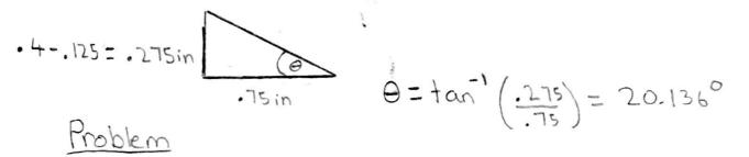
I want to <u>maximize</u> the amount of <u>axial loading</u> to <u>avoid bending</u> by increasing the angle,  $\Theta$ . However the forbidden Zone is in my way and the position of the hole can't be moved. If I reduce the amount material around the hole, its more likely to break due to <u>Small</u> cross sectional [dea
